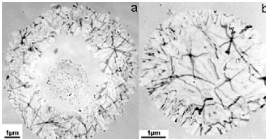
FIG. 2. Different structure of the crystallised spot in  $\text{Ge-Sb}_2\text{Se}_3$  bilayer resulted from different e-beam intensity (a – stronger)
